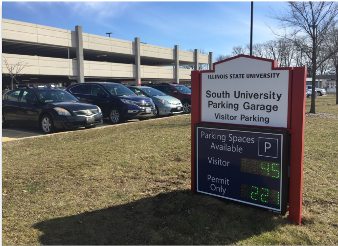
Variable Message Sign (VMS) Conveying Real-Time Data to Drivers
