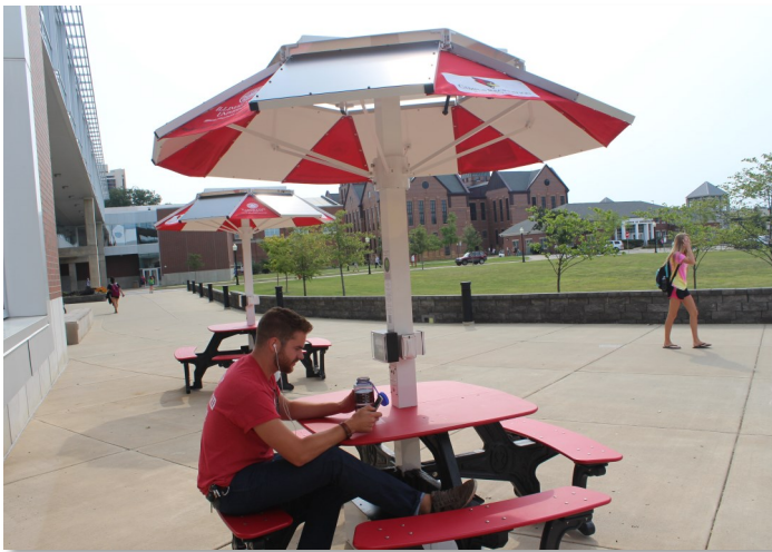
Solar-Powered Charging Stations at Student Fitness Center
